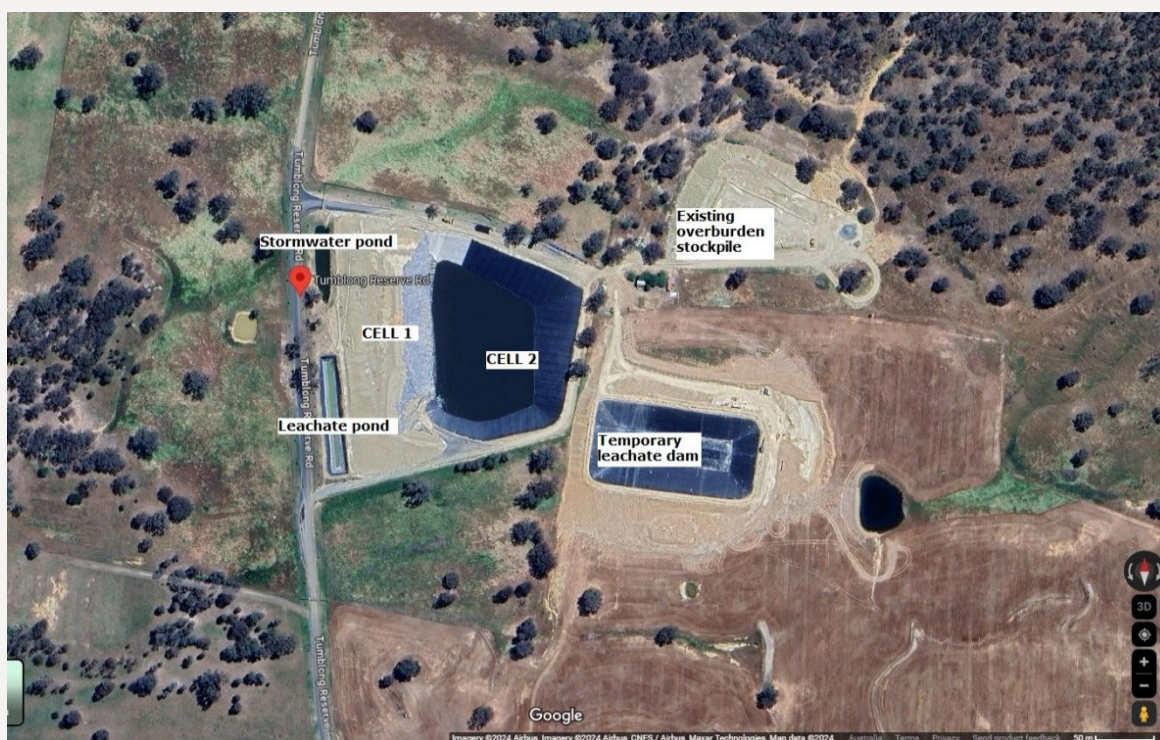
Figure 1 | Annotated Landfill Aerial
